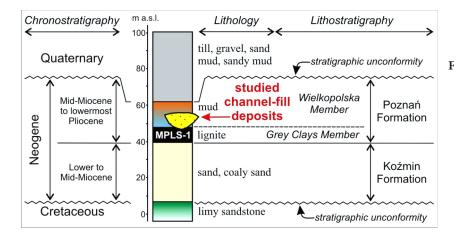
Fig. 2. Stratigraphical sketch of the Cenozoic succession within the Kleczew Graben (modified from Widera, 2007, 2014). Note the stratigraphical position of the examined channel-fill deposits within the muddy Wielkopolska Member of late Neogene age; MPLS-1 – the First Mid-Polish lignite seam; for approximate position of the lithological section see Figure 1C
