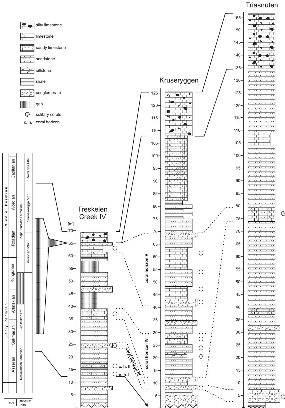
**Fig. 3.** Correlation of Early Permian (Early Sakmarian) rock units from the inner Hornsund area. Stratigraphic sections without the older layers of the Treskelodden Formation from which rugose corals have not been ascertained. Approximate total thicknesses: 100 m for Treskelen, 150 m for Kruseryggen and 180 m for Triasnuten (based on Nowak, 2007, modified).
